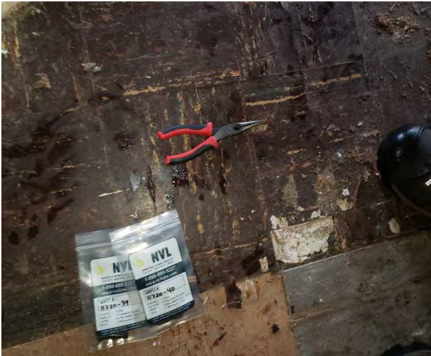
Photo #5: Samples 11720-39 & 40: 9"x9" Brown VFT on black mastic (on wood.) (9% Chrysotile) Location: Building 9 Main Floor
