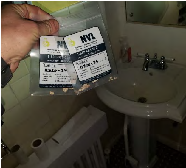
Photo #3: Samples 11720-24 & 25: 4'x4' cream ceramic tile with gray grout (on plaster.) (4% Chrysotile) Location: Building 8 Entryway Bathroom
